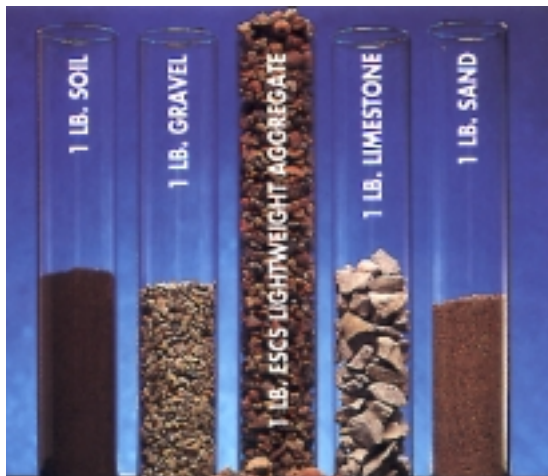
Lightweight Aggregate offers more than twice the aggregate volume for the same weight of conventional aggregate.
